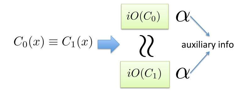
Functionality preserving: the functionality of a circuit does not change after being obfuscated.
